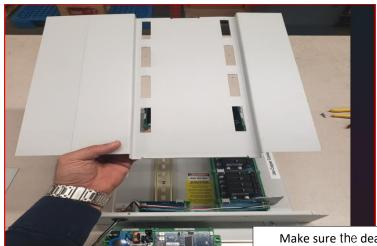
Make sure the dead front cover will lay down under the edge of the horizontal voltage barrier.
