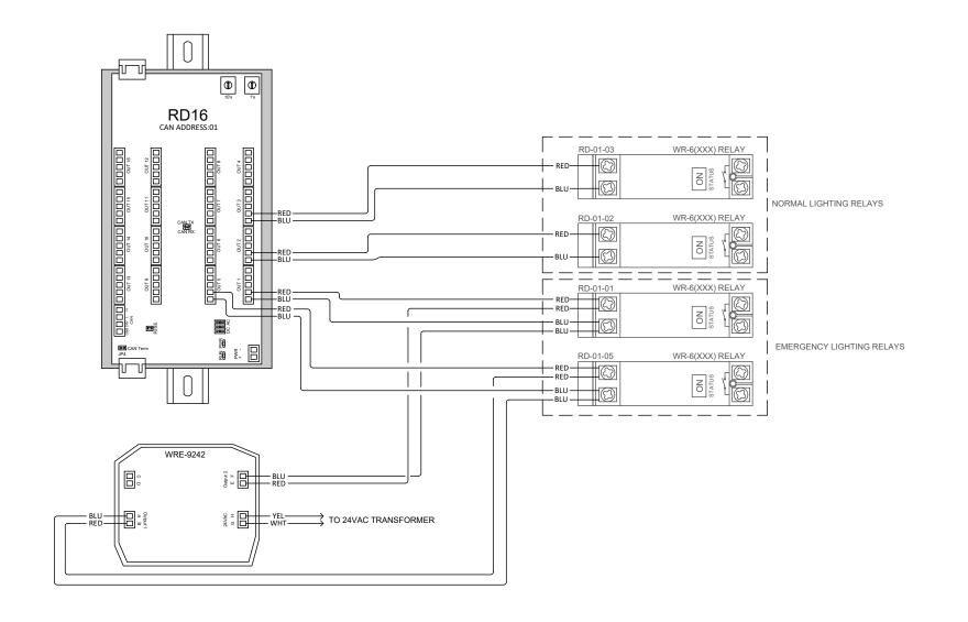
The Douglas WRE-9242 Emergency Relay Driver provides UL924 emergency switching capabilities for up to two Douglas WR-6xxx relays.
