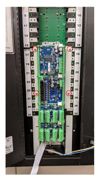
4) Once the RK has been mounted in the panel, begin connecting the wiring according to the wiring typical and specifications. All connections, except the ribbon cables, from LMB & LX5/LX6 controller board will need to be re-terminated to the RK modules.
