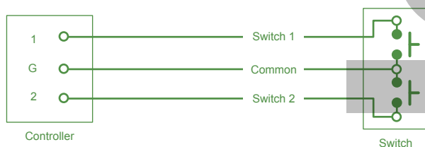
Digital Input: Two Button Low Voltage Switch (Dry Contact)
