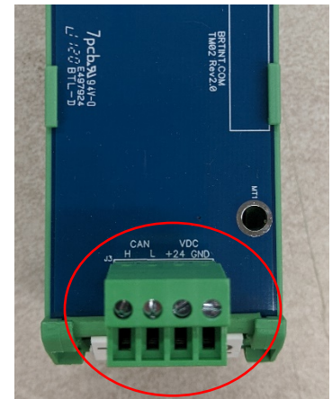
Photo of TM02 with CANbus Terminal
