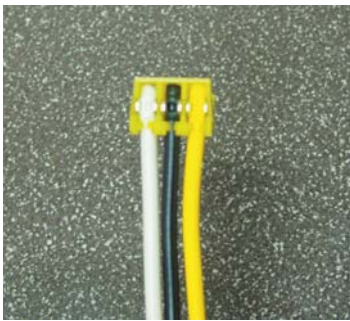
Proper wire order after crimping
